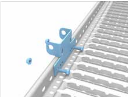
Mount the WFANDL start and end fastener at the beginning and end of the wire strand. Installation takes place with the 2 bolts and nuts from bolt set 32..
