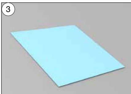
3 Cut a minimum 800 x 900 mm rectangle of the membrane.
